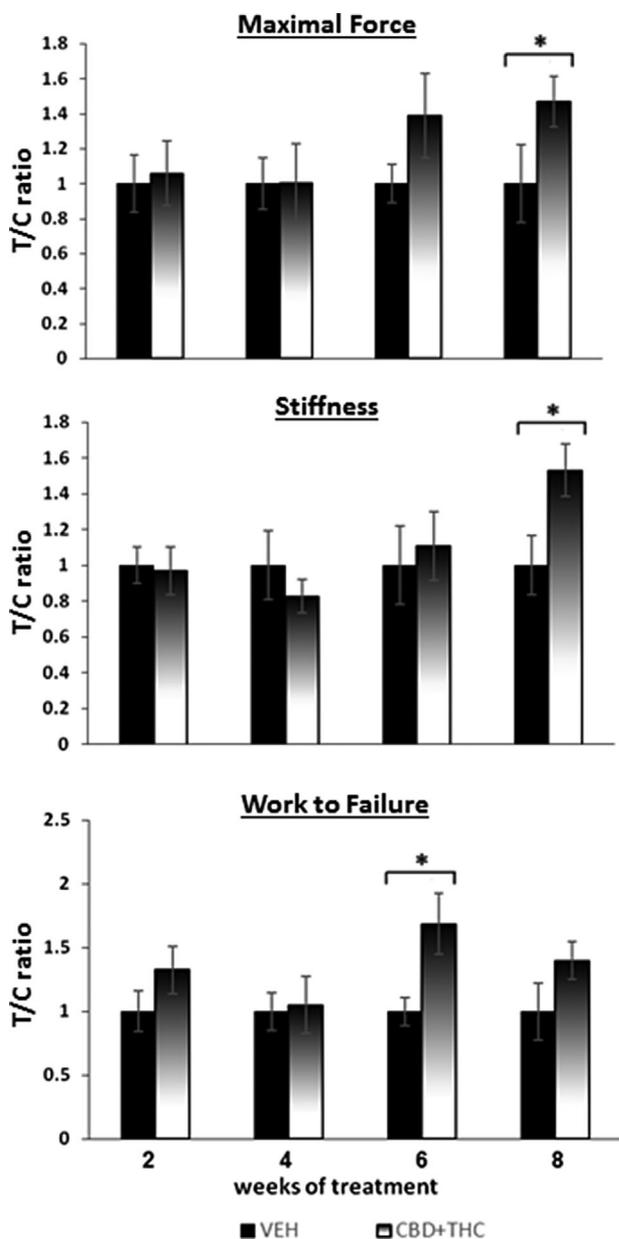
**Fig. 4.** Effect of THC-CBD mixture on fracture callus biomechanical properties. Data are mean  $\pm$  SE obtained in 8 to 13 rats per condition. \* $p < 0.05$ . VEH = vehicle; CBD = cannabidiol; THC =  $\Delta^9$ -tetrahydrocannabinol; T/C ratio = THC/CBD ratio.
