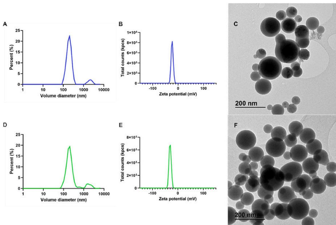
Fig. 1. Characterization of PBS nanoparticles (blank: A-C; and CBD-loaded: D-F): volume diameter distribution (A, D); zeta potential distribution (B, E) and TEM images (C, F).
